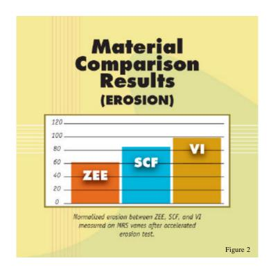
ZEE generated fewer particulates than competitive materials Components manufactured from ZEE showed less weight loss than SCF or VI components. (See Figure 3)
